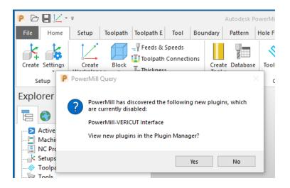
Click File tab > Options > Manage Installed Plugins to display the Plugin Manager dialog where you can manage the plugins that are installed on your PC. Select the PowerMIII-Vericut Interface and pick Enable
